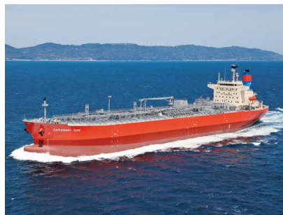
World's first methanol tanker equipped with a methanol-fueled main engine
